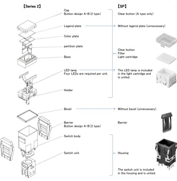
The SP integrated P/N will differ depending on the combination of the Series 2 components. Please confirm what kind of combination is used, please convert the integrated P/N to the SP.
