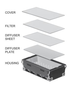
※ For a colored filter, if the positions of the diffuser plate and filter are reversed, the luminescence will be soft color.
