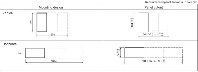
💥 If the panel is to be finished (e.g. coated), make sure that the panel meets the specified dimensions after the coating.
