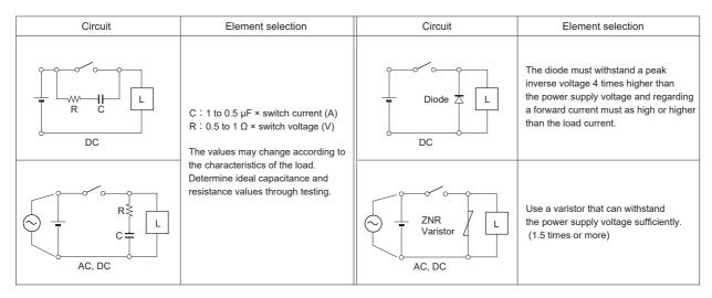
(9) Following circuits show examples of an anti-chattering circuit.
