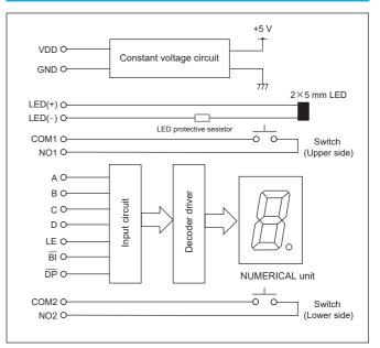
% DC 5 V, DC 12 V input type does not have a built-in constant voltage circuit.
